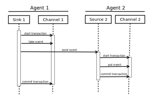
A Transaction is implemented within a channel implementation. Each source and sink that is connected to channel must obtain a Transaction object. The sources actually use a channelselector interface to encapsulate the Transaction. The operation to stage an Event (put it into a channel) or extract an Event (take it out of a channel) is done inside an active Transaction. For example:
